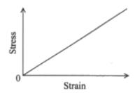
Show that the area under this graph represents the work done per unit volume in stretching the sample.
